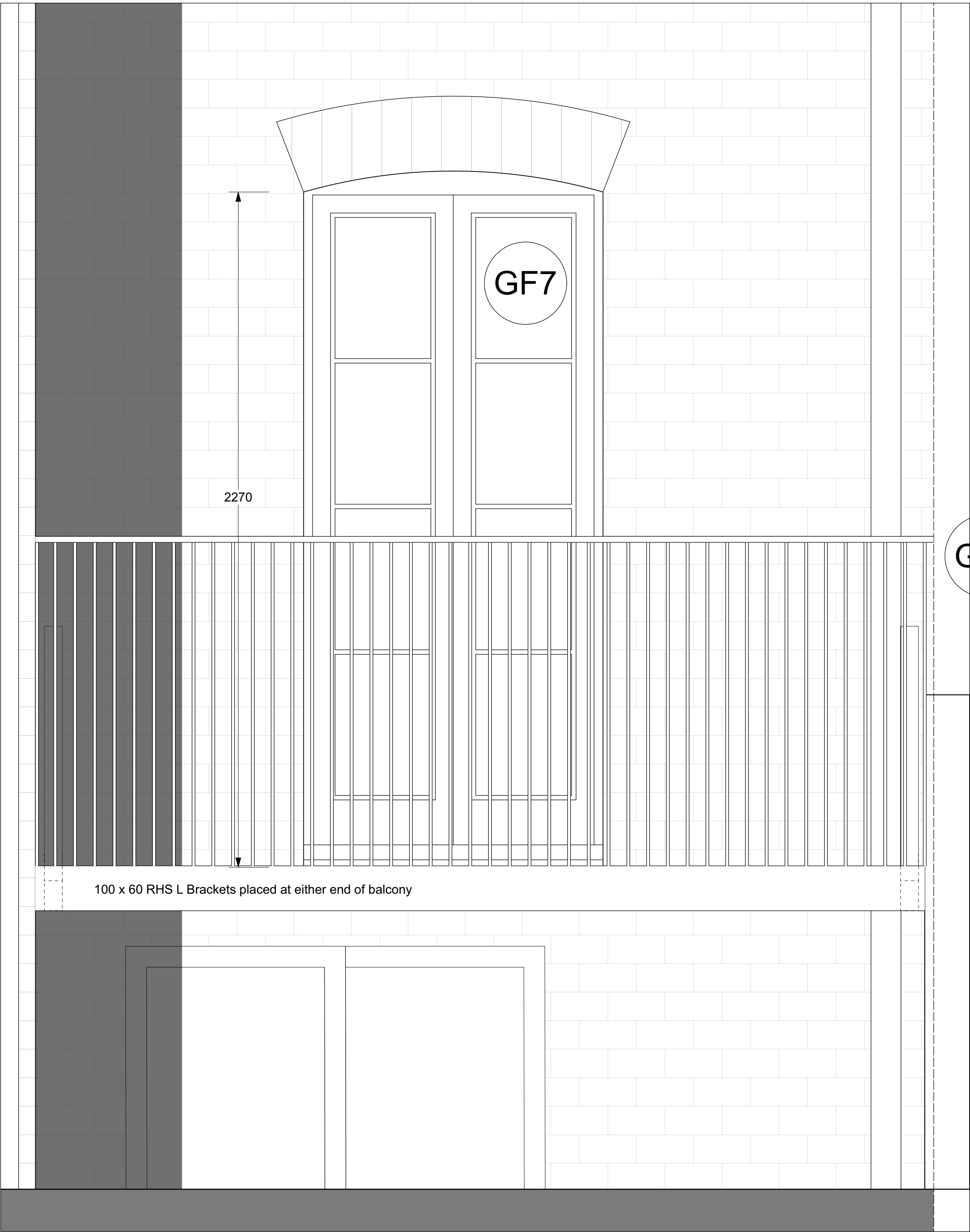
Rear Elevation of Balcony & Rear French Door 1:10
