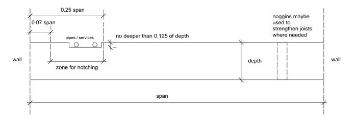
TRADA (The Timber Research and Development Association) and BS5268-2 guidance on how large holes and notches can be cut out of standard floor joists, and still remain within safe working limits.
