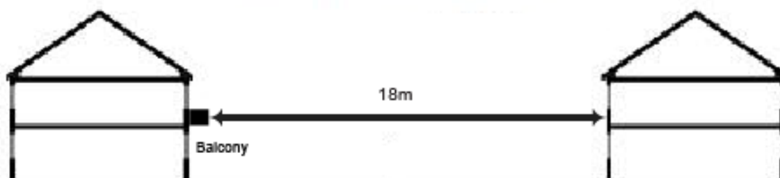
Figure A: 18m separation distance measurement
