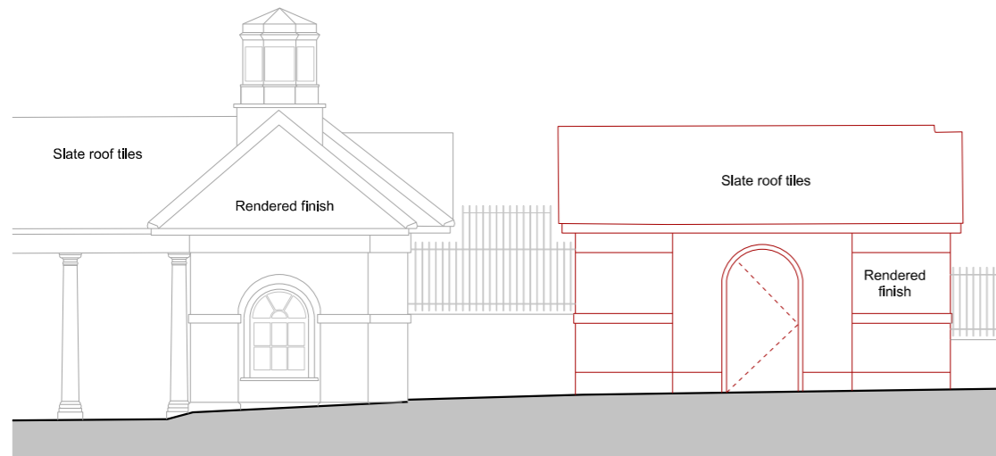
Existing West Elevation A-A
