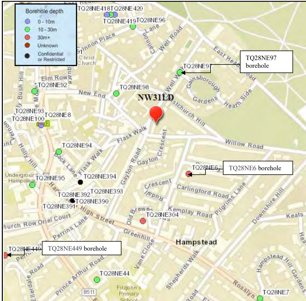
Figure 14 Local Borehole Plan
