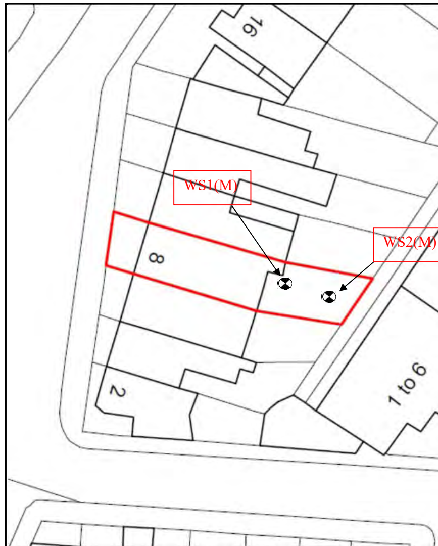
Figure 27 Borehole Location Plan
