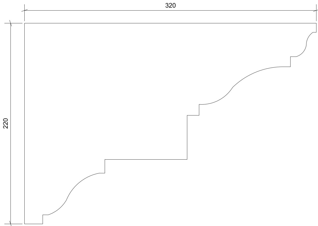
01 A6900 Cornice Type A Proposed typical ground floor cornice profile rG.02 rG.03
