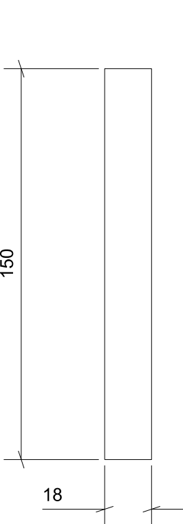
05 A6900 Skirting Type A Proposed typical lower ground floor skirting profile rLG.01 rLG.02 rLG.03 rLG.04 rLG.05 rLG.07
