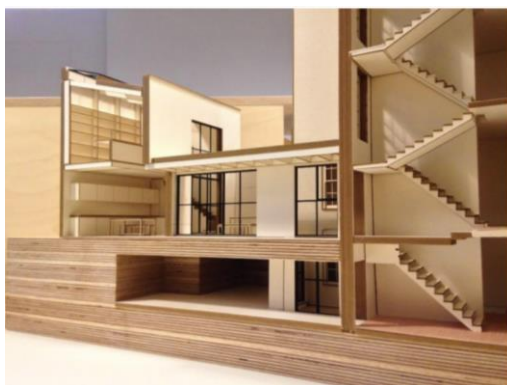
Figure 15: Model showing approved (2015/7223/P) works to the rear annexe at no.36 Great James Street including mezzanine to first floor and large, double height window opening on the front elevation and the full length skylight in the roof
