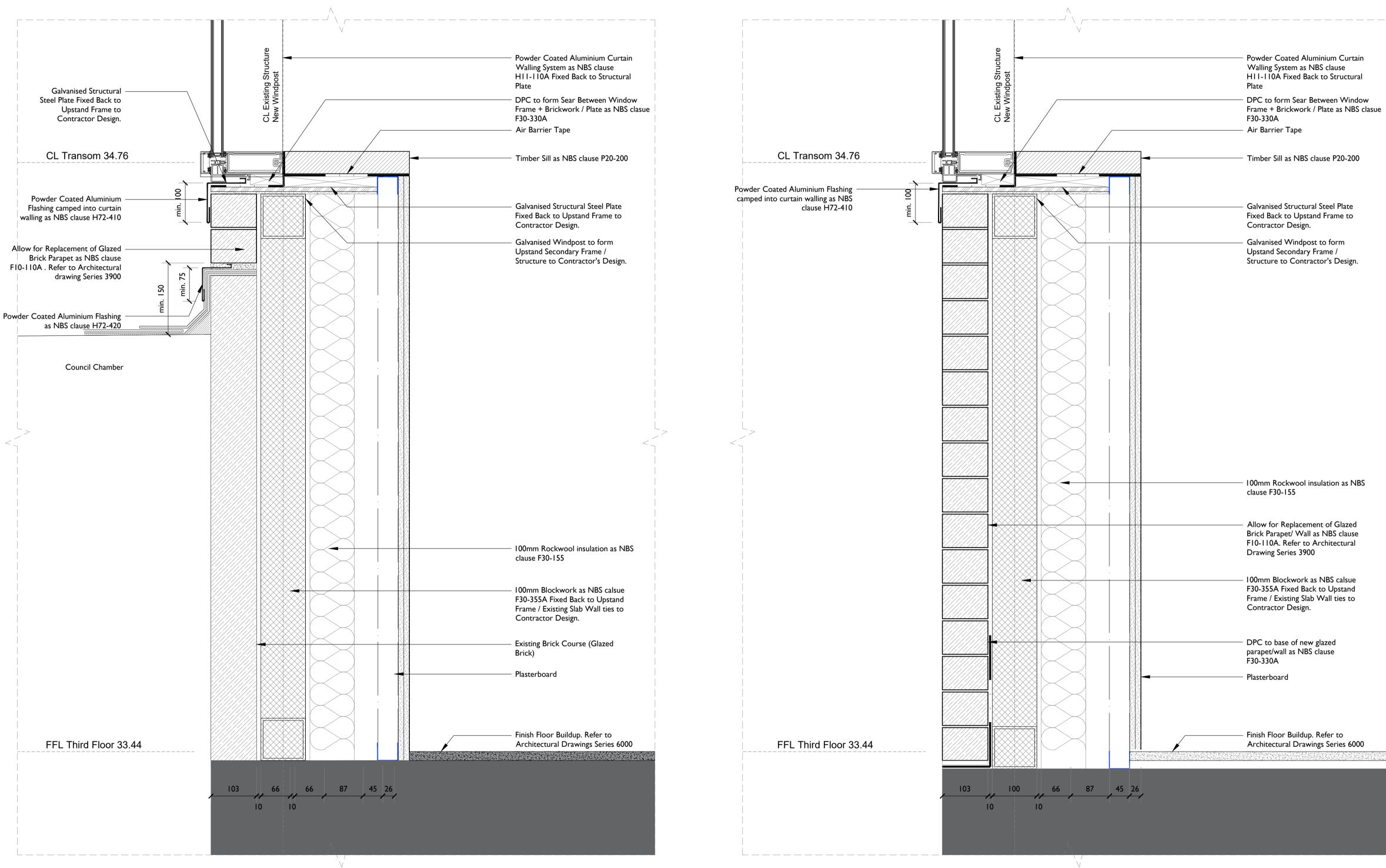
**CURTAIN WALL PARAPET TYPE 3** 6207 I:5 @ AI
