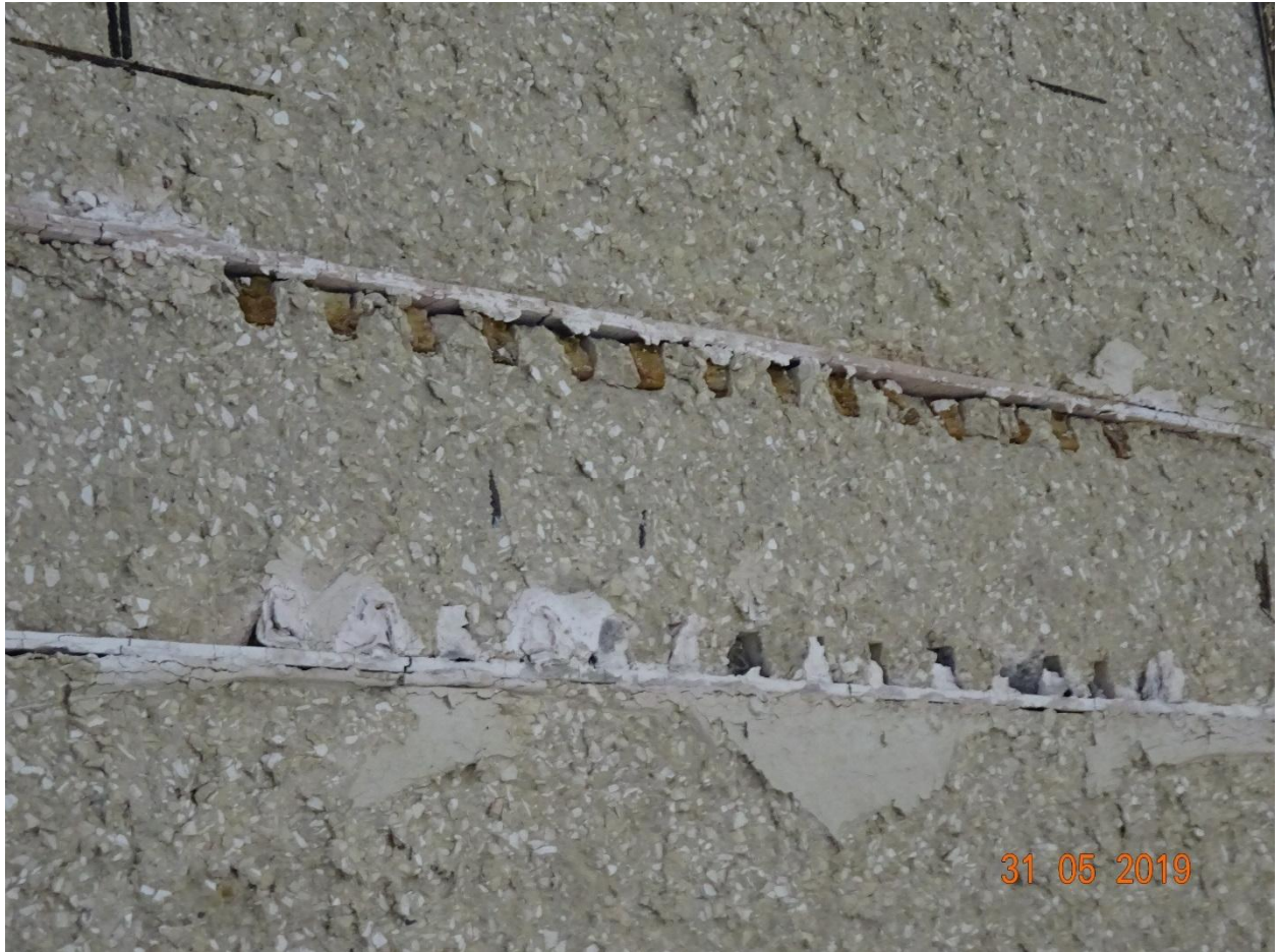
Photograph 6: Exposed face (fireside) face after test.
