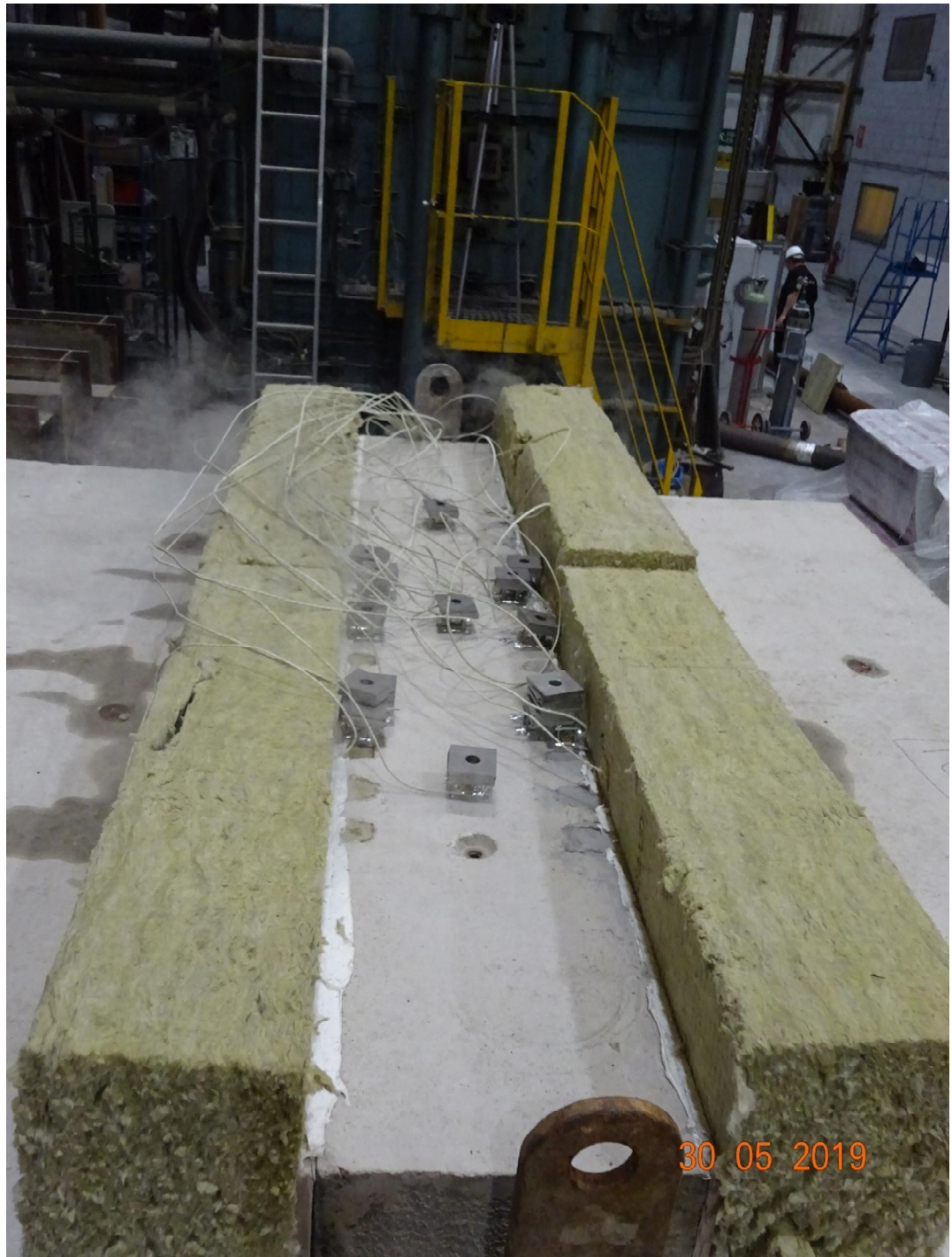
Photograph 5: Unexposed face (non-fireside) face after 60minutes from the start of the test.
