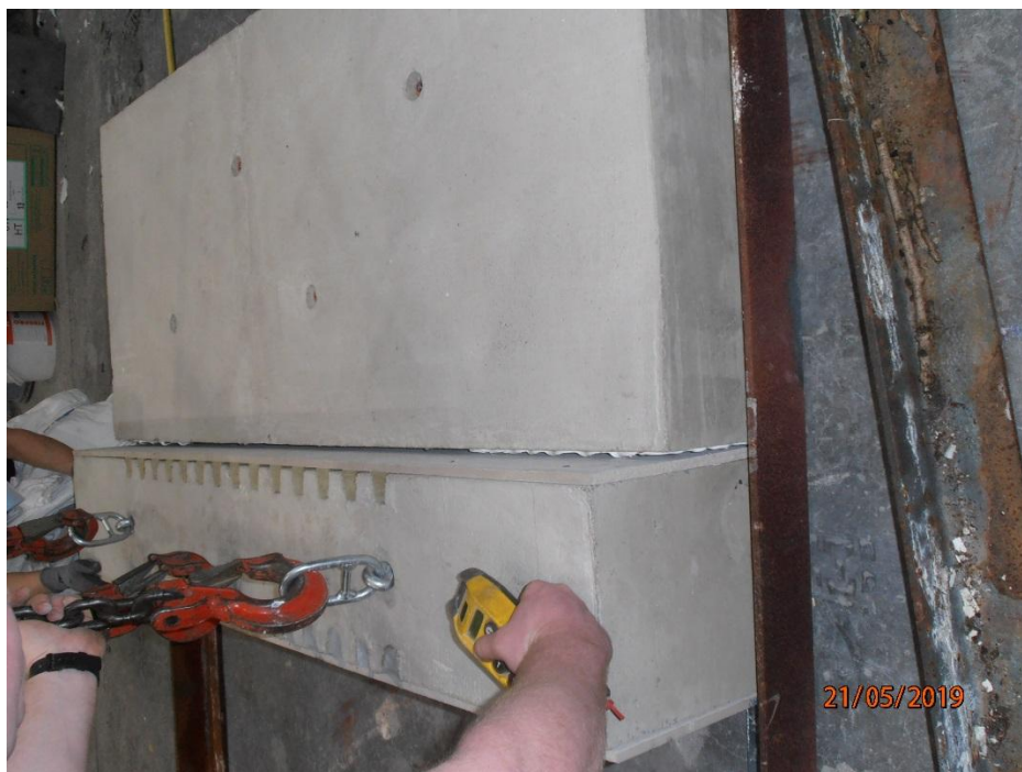
Photograph 2: Installation of test specimen into test frame.
