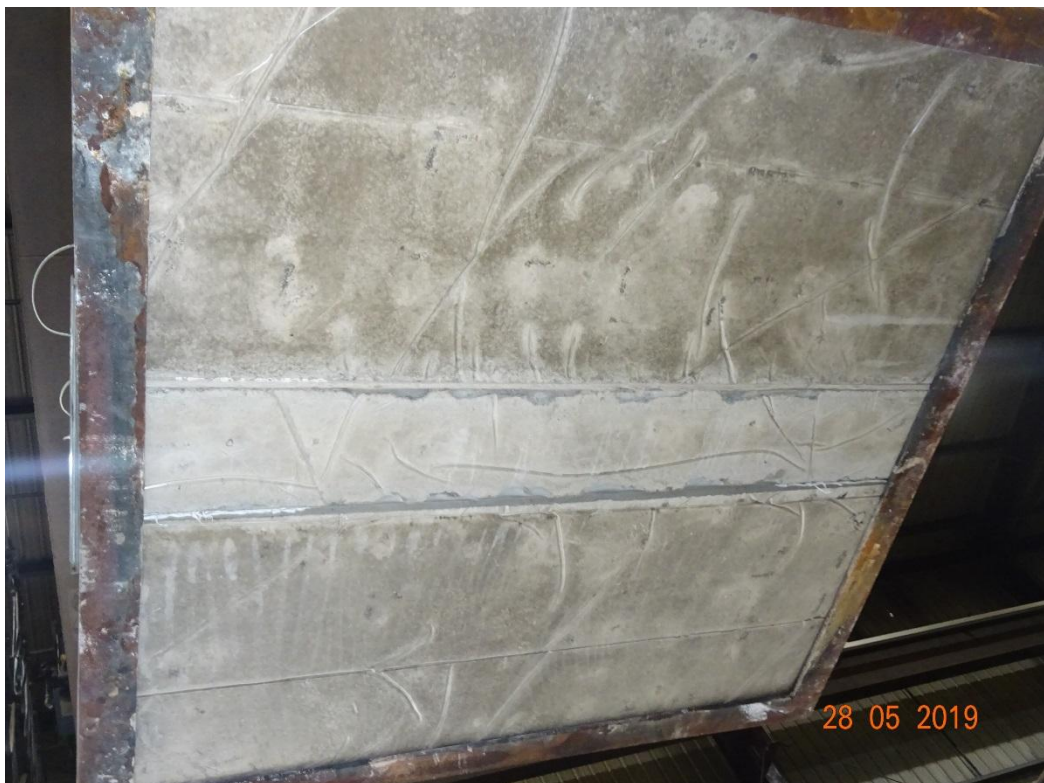
Photograph 5: Exposed face (fireside) face before test.
