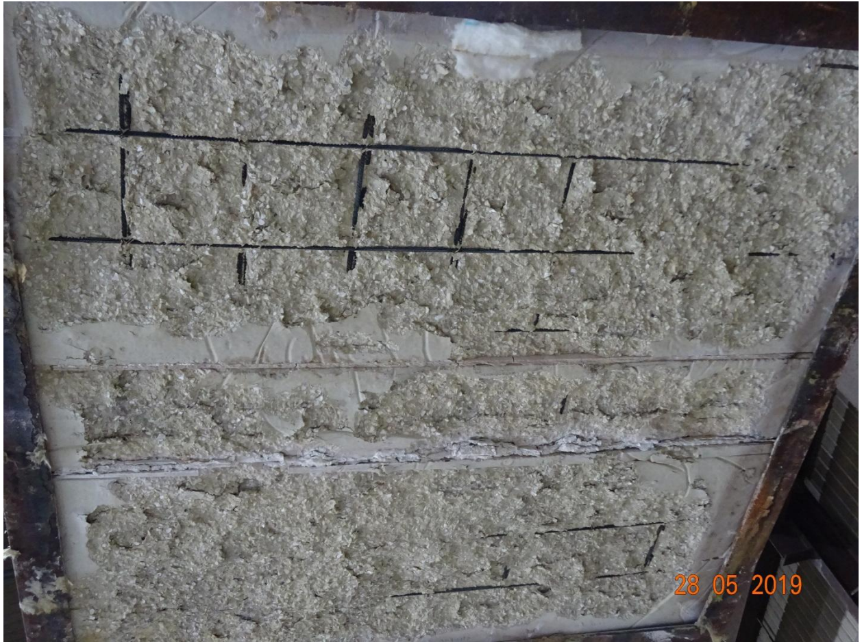
Photograph 7: Exposed face (fireside) face after test.
