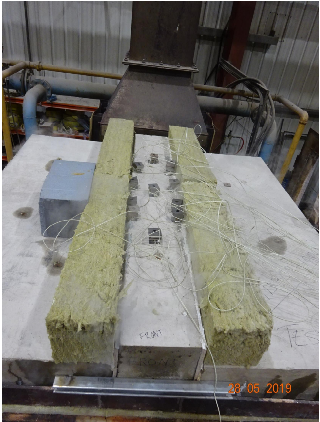
Photograph 6: Unexposed face (non-fireside) face after 60minutes from the start of the test.
