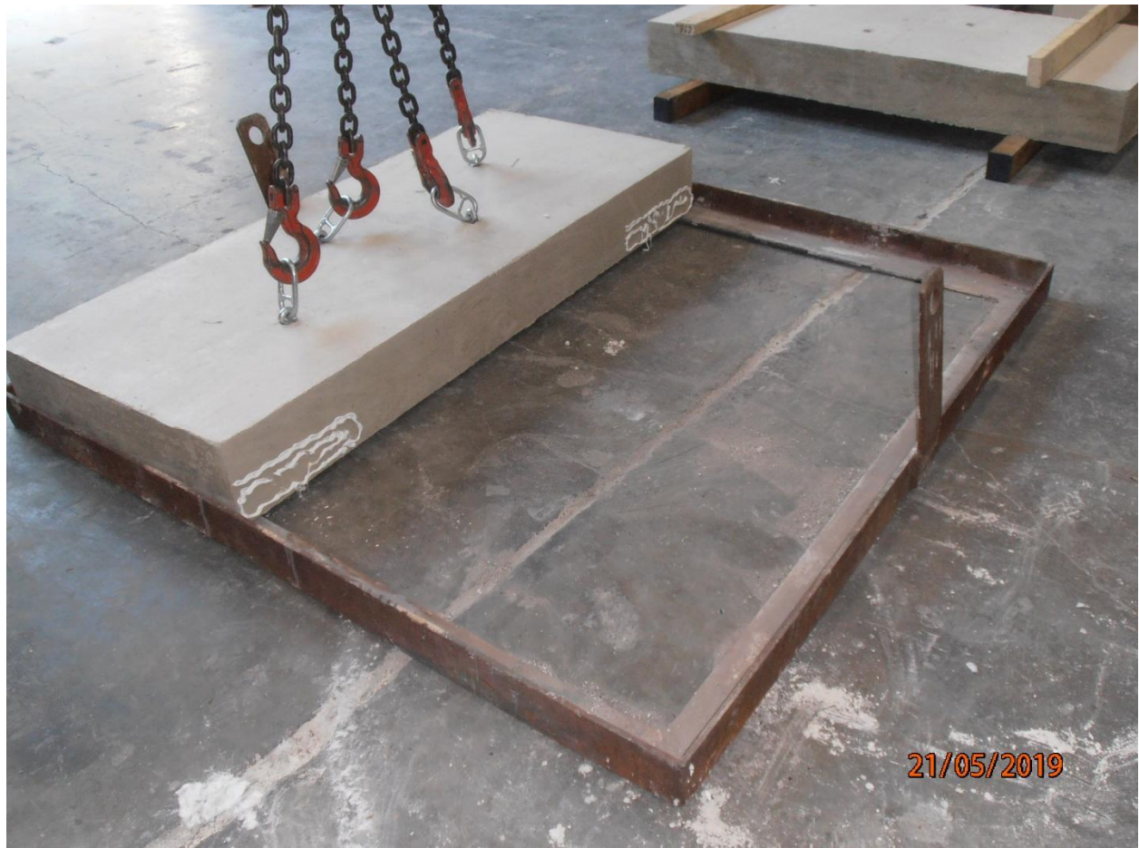
Photograph 1: Installation of specimen into test frame.
