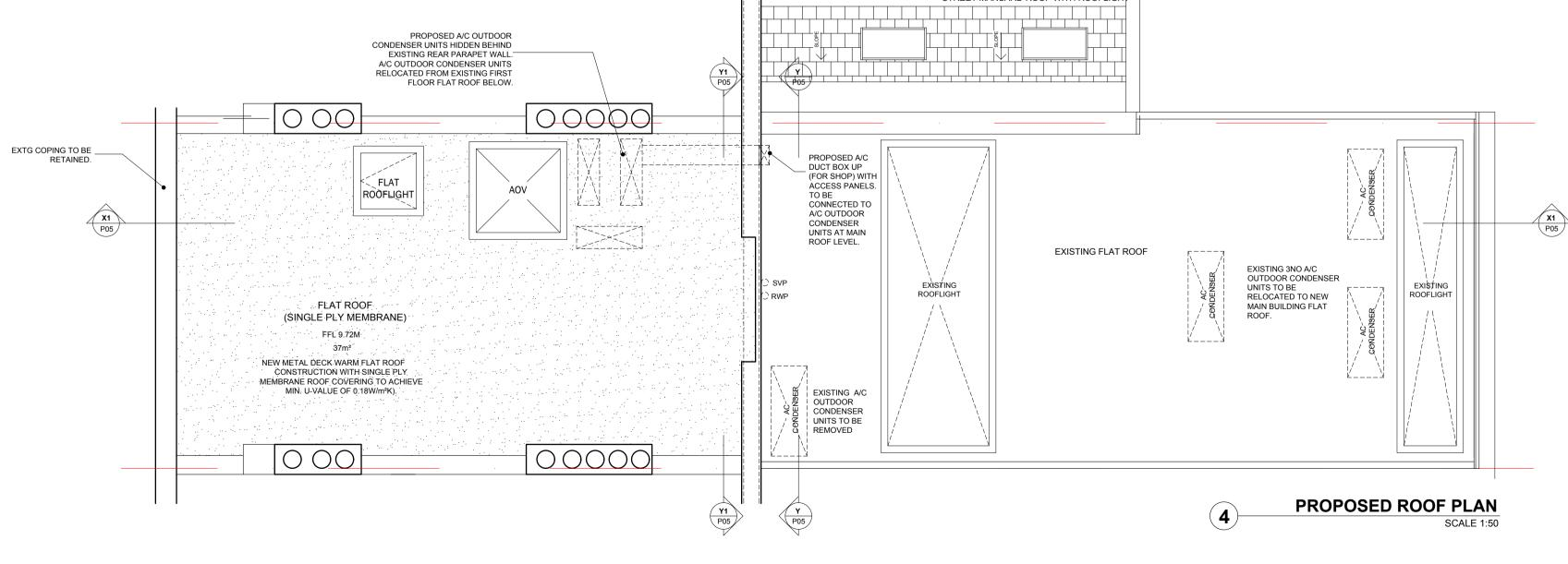
General Notes: Revisions: B 15.01.21 AC DUCT ON REAR ELEVATION 1. Please do not scale from this drawing. 2. All dimensions to be checked on site by the contractor. INDICATED All references to drawings refer to current revision of that drawing. Structural services information shown is indicative only. Refer to consultants drawings for details and setting out.
