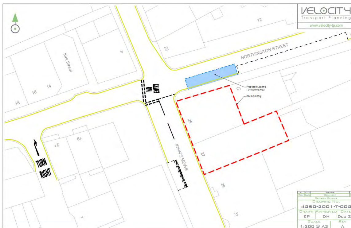
Figure 4-3: Site Set Up Plan – Excavation and Underpinning Phase
