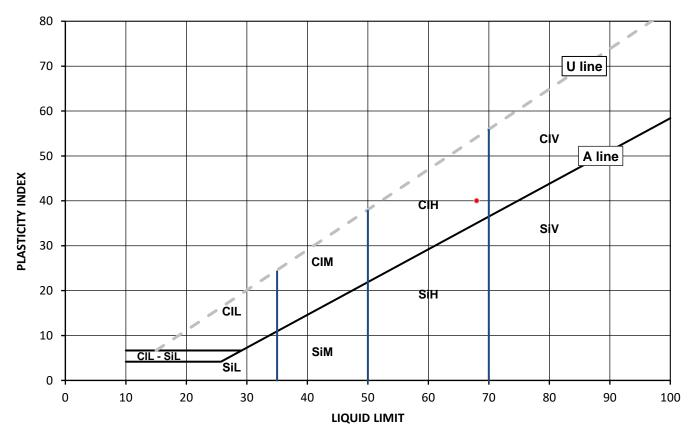
Legend, based on BS EN ISO 14688 2:2018 Geotechnical investigation and testing - Identification and classification of soil
