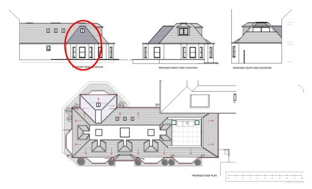
4) Amended proposed plans/elevations uploaded to Camden Council's website 21/12/2020 (with clearer plans of the same proposal uploaded January 2021). Note the ridge of the rear projection (subject of this application) finishes 400mm below the main roof ridge. This is an overall increase of 600mm above the existing situation shown in image no.2 above.
