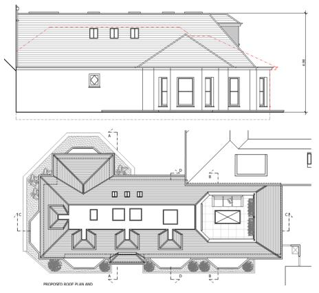
2) Existing plans as previously approved under ref: 2017/4730/P dated 21/11/2017 and implemented in 2020. Note the ridge of the rear projection (subject of this application) finishes 1m below the main roof ridge.
