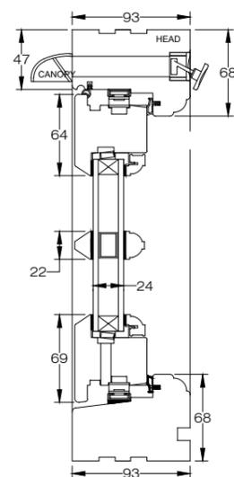
Typical white painted timber casement window in conservation area style. Double glazed toughened glass with white smooth warm edge. French opening panel(s). All items to comply with building regulations including Part B (fire regulations and Part K (impact and collisions)
