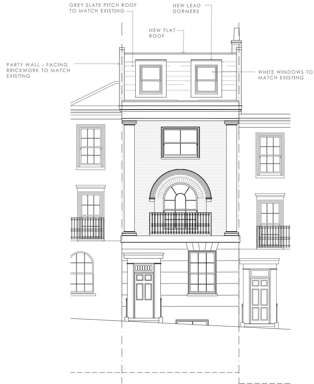
PROPOSED FRONT ELEVATION SCALE 1.100
