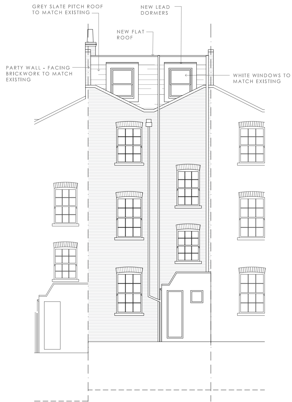
PROPOSED REAR ELEVATION SCALE 1.100
