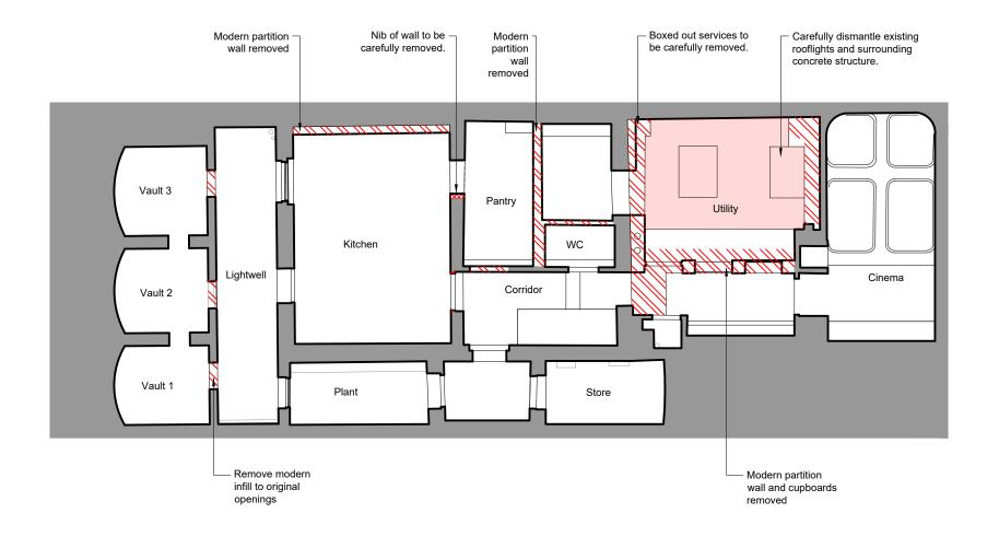
01 Basement Reflected Ceiling Plan 5500 1:100 @ A3 Load bearing walls to be removed
