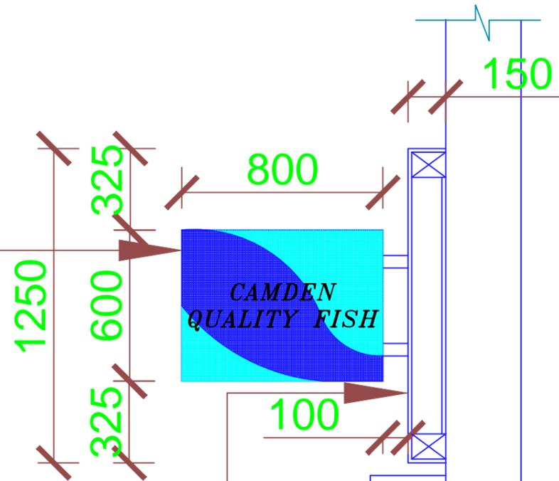
1 no. Proposed new internally illuminated fasica sign to consist of individual built up letters and logo with internal L.E.D illumination. illuminated letterset and logo to be mounted on PPC aluminium backing , finished in Blue.
