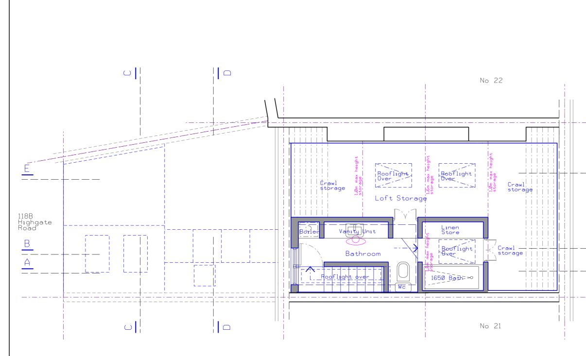
Proposed Loft Floor Plan Scale 1:50
