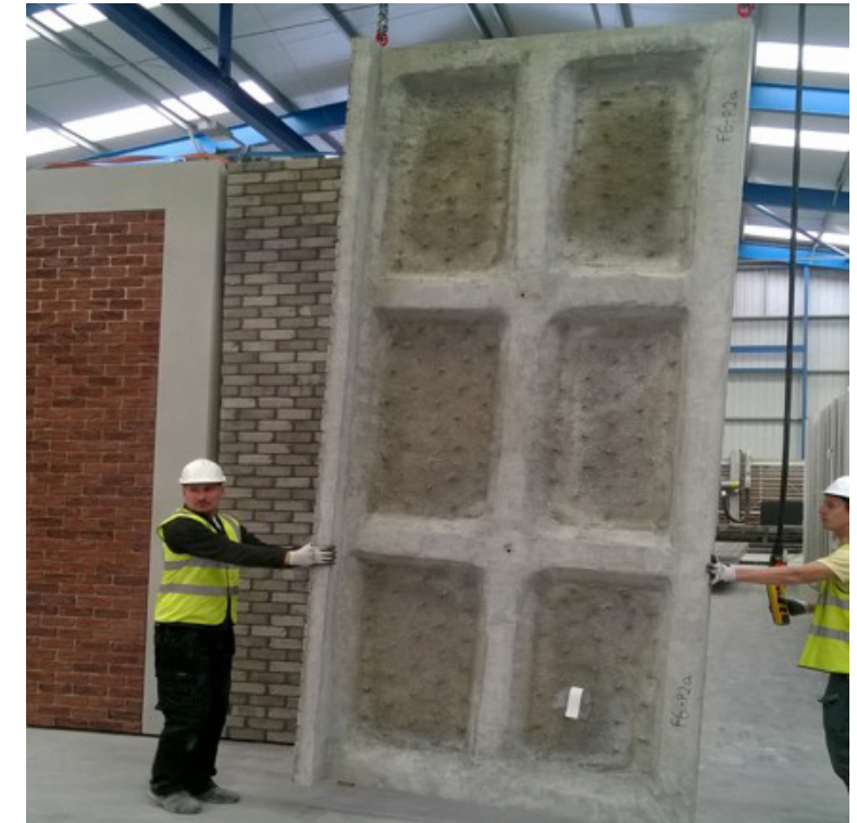
Reverse side of GRC backing
