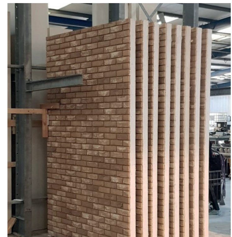
The depth of the GRC backing makes each panel robust
