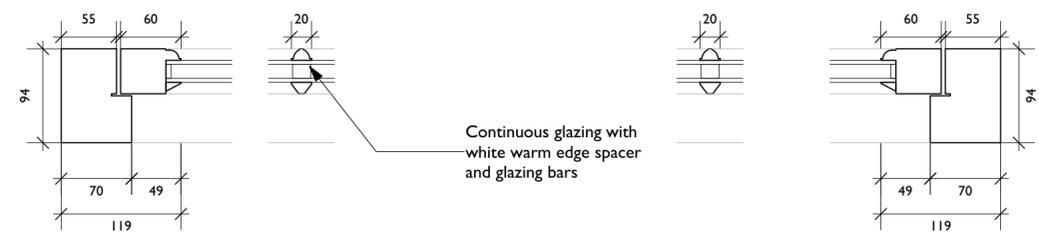
Continuous glazing with white warm edge spacer and glazing bars
