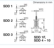
Rubber elements are suitable for small to middle weights and ambients up to + 60 °C. Spring elements are suitable for higher temperatures above + 60 °C (e.g. smoke extraction).
