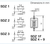
Important note for installation! Make sure that fan system is well balanced (centre of gravity of heavy motor may cause uneven loading of mounts).
