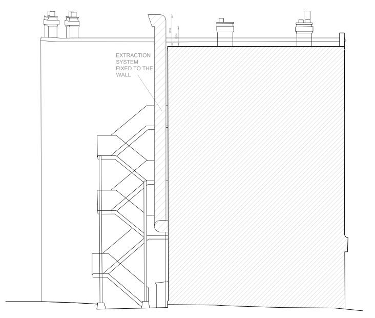
Proposed Left Side Elevation Scale 1:100
