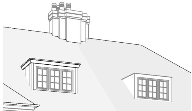
Option 3: Existing and Proposed view of roof and dormer windows, showing raised dormer roof and thicker cheeks with indicative detailing.
