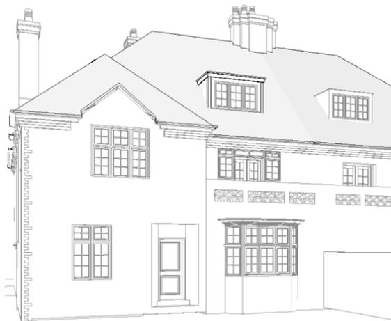
Option 3: replace tiles, keeping to same roof height – note new tiles will have a slightly different appearance.
