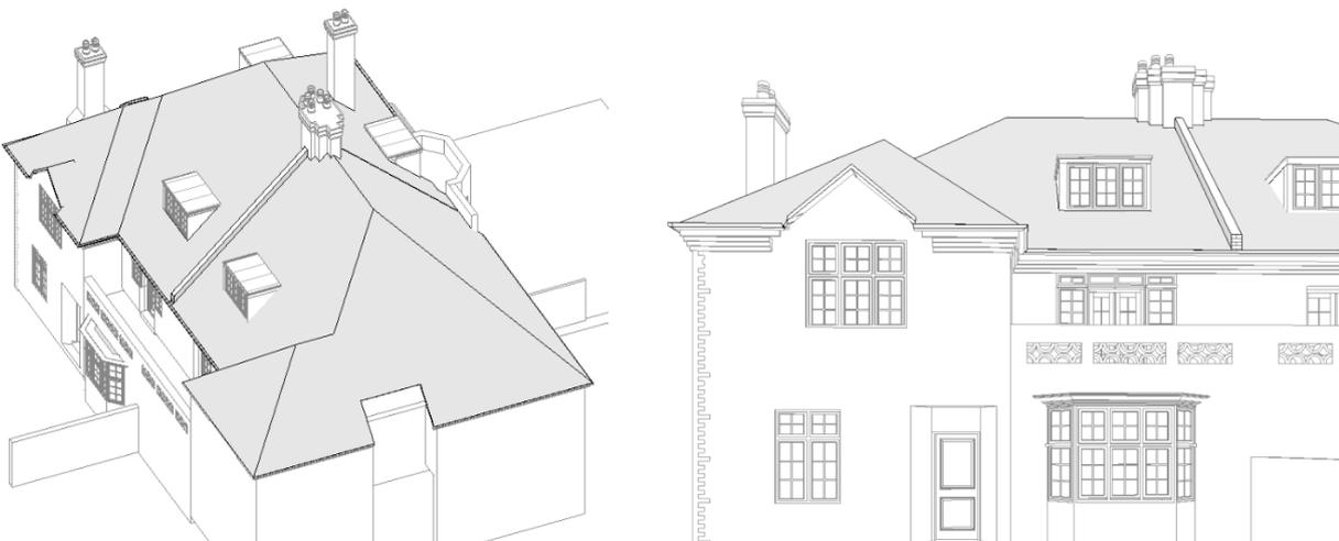
Option 2: Build a parapet wall at the front over the party wall to mask the change in level and any difference in the appearance of new and old tiles
