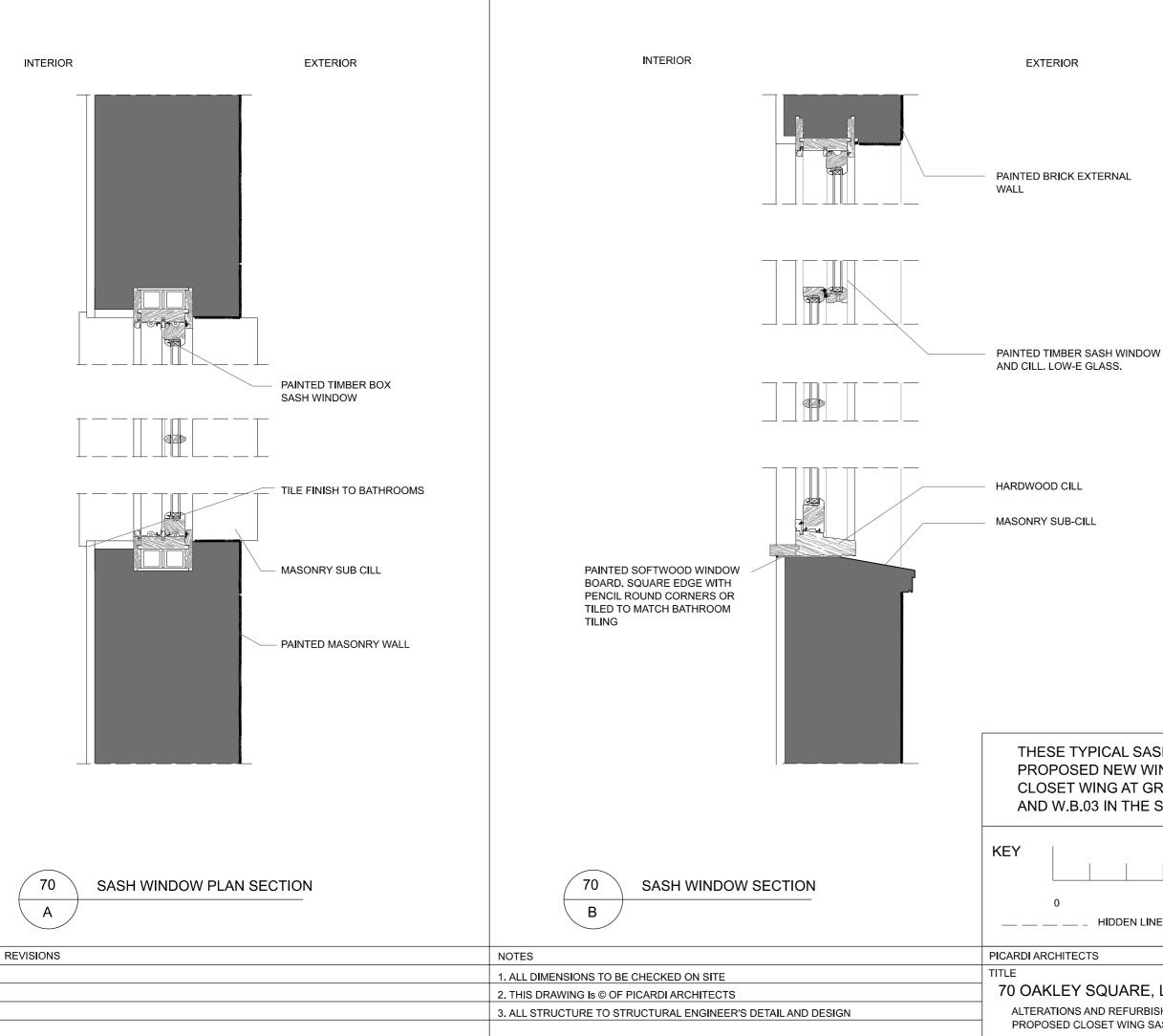
THESE TYPICAL SASH WINDOW DETAILS APPLY TO THE PROPOSED NEW WINDOWS W.G.06 AND W.B.05 IN THE CLOSET WING AT GROUND AND LOWER GROUND FLOORS AND W.B.03 IN THE SIDE LIGHTWELL.
