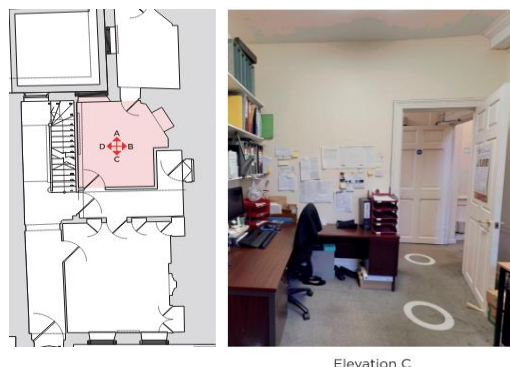
Figure 15 showing current ground floor rear room divided with corridor accessing no.7 Great James Street.
