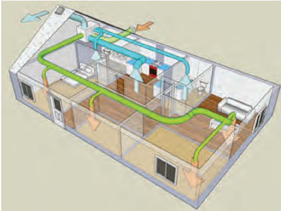
Residential whole house ventilation system
