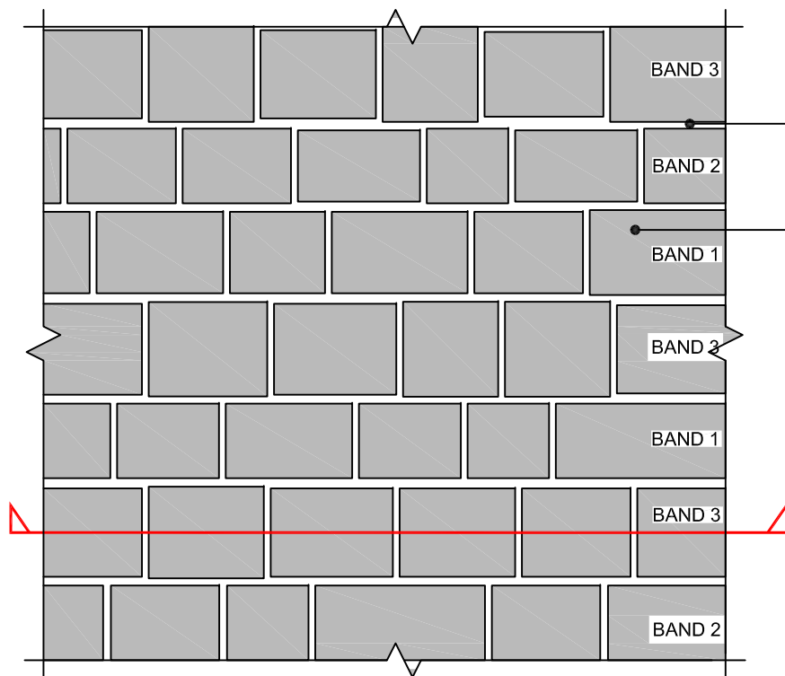
DETAIL H06a - PLAN LAYOUT OF PAVING TYPE 6: RECLAIMED GRANITE SETTS SCALE 1:10 @ A3
