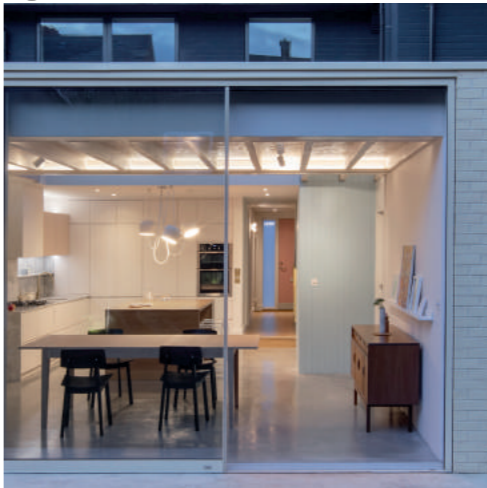
Thin framed double glazed aluminium sliding doors & thin profile powder coated aluminium cappings
