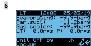
The status on the front screen will now indicate “Unit OFF by vacuum”, in this state the CDU cannot be set in ON.
