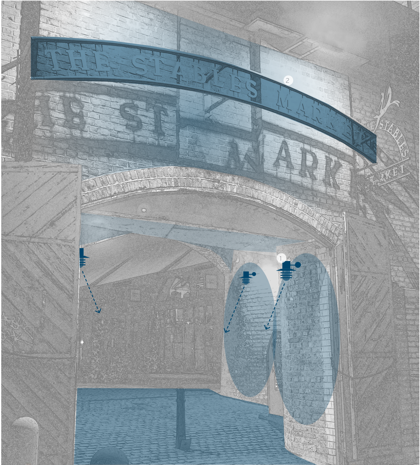
Shielded wall mounted luminaires to reduce glare and provide amenity lighting to the passage way. Decorative shade and bracket design to be designed with the architectural team.
