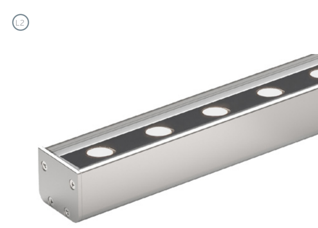
Location: Terrace planters Manufacturer/Product: Lightgraphix/ LD38 Specification: Warm colour temperature, oval or narrow beam distribution luminaire fixed at the back and front of key planters to graze the back panels and highlight the feature vegetation. Supplied with cowl and anti glare louvres; 17W/m, 1480lm/m
