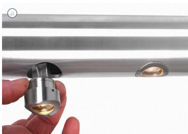
Location: Ramp Manufacturer/Product: Stoane Lighting/ Indehandrail Module Specification: Warm colour temperature, soft asymmetric distribution luminaires for recessed installation in handrail profile; 4W/m, 171.6lm/m
