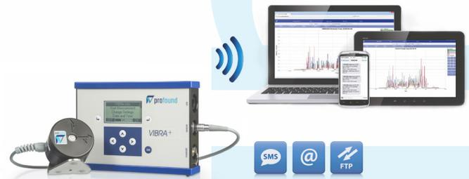
An alarm level can be set for velocity whereby an external wireless alarm beacon can be used to warn on-site and remotely via SMS. The *VIBRA*<sup>+</sup> model also features a smart frequency-dependent velocity, acceleration and displacement alarm, and can send alerts via SMS and e-mail.
