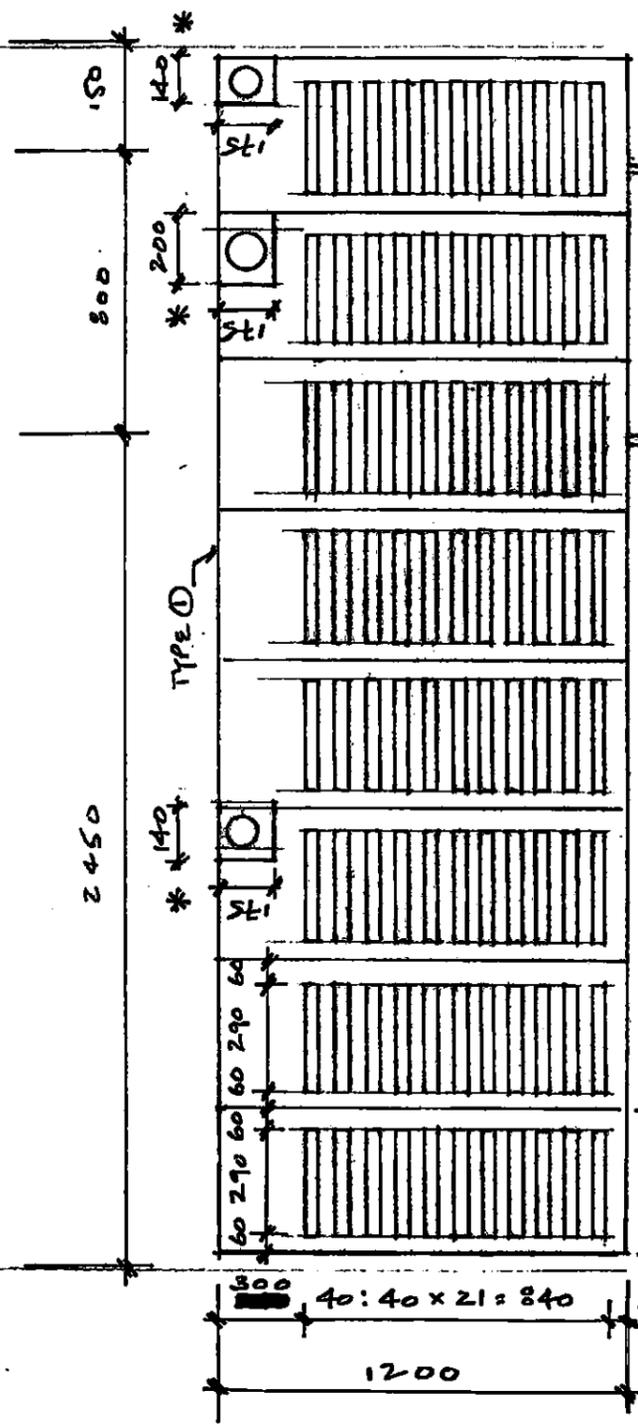
SLOTTED 20mm MS PLATE 40mm SLOT: 40mm SOLID. LAZER CUT. TO DETAIL DRAWING.
