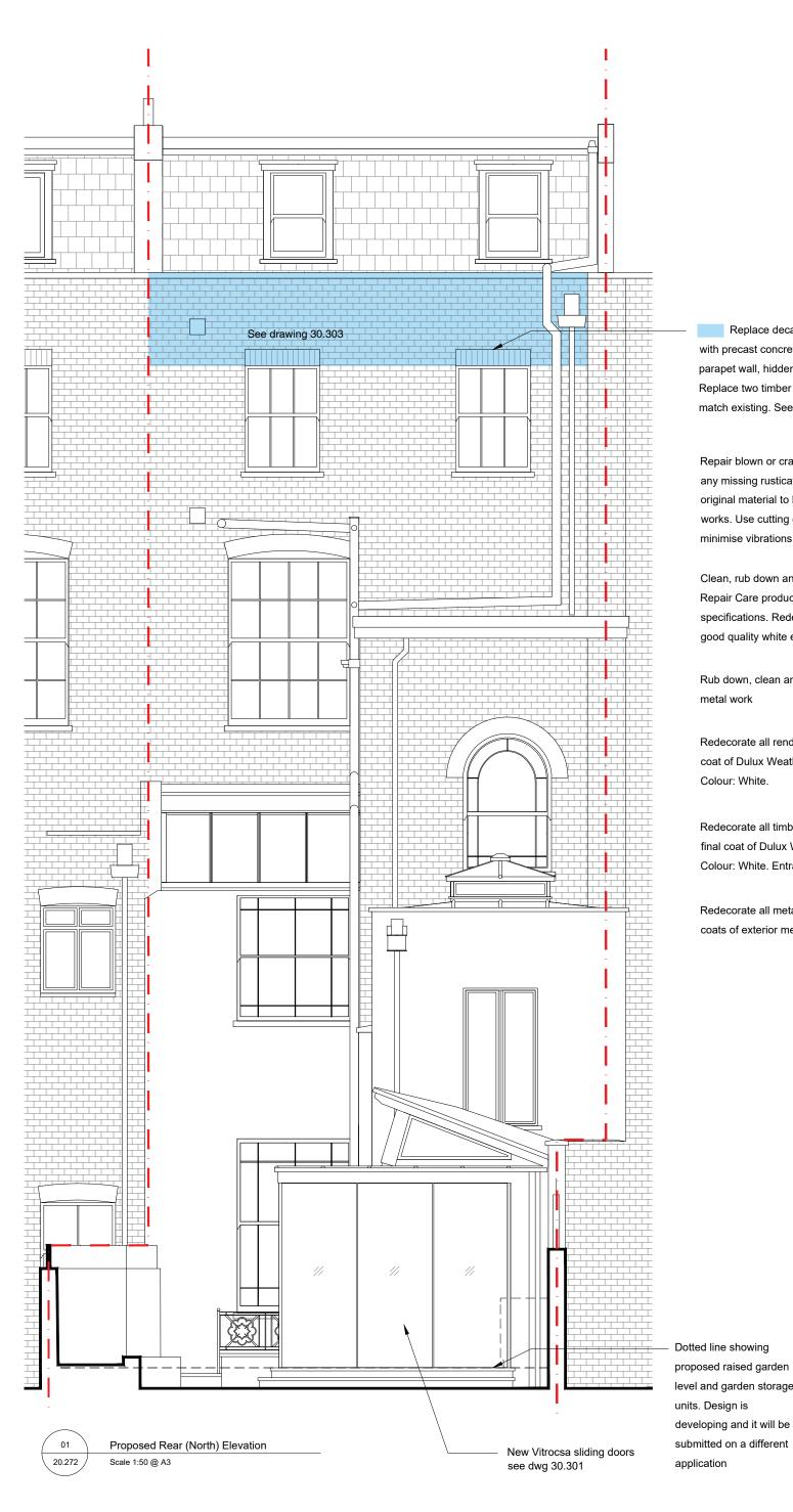
Replace decayed wooden lintels above windows with precast concrete lintels as per SE details. Rebuild parapet wall, hidden gutter detail and replace coping stone. Replace two timber sash windows - size and design to match existing. See drawing 30.303
