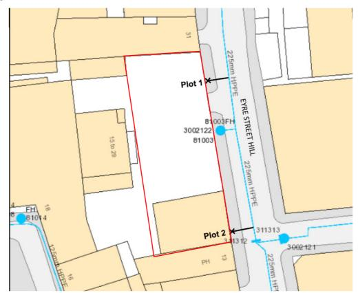
The test confirmed that the maximum water flow achieved was 1,800 litres per minute at 2.9 bar pressure.
