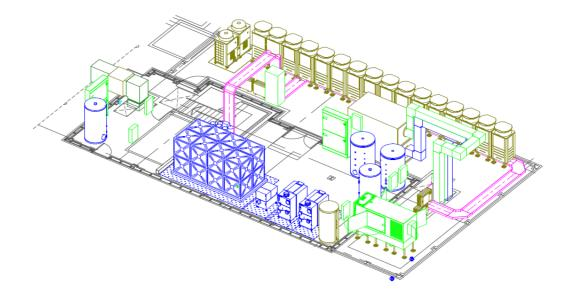
To protect the hotel in case of disruption in water supply from the mains network the incoming cold water mains has been sized allowing for replenish the tank in approximately 2 hours.
