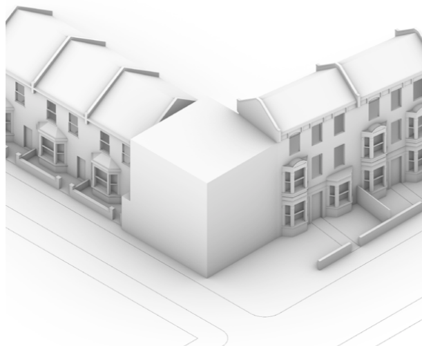
Extrusion of existing plan with set back between terraces
