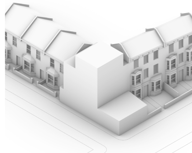
Extending to front at ground floor and providing additional loft level for extra bedroom.
