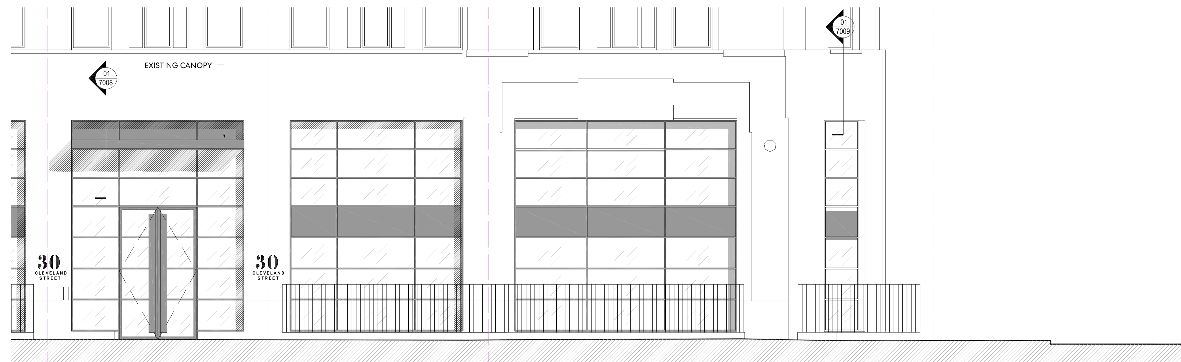
3 ENLARGED EXISTING SOUTH-WEST ELEVATION 1:50
