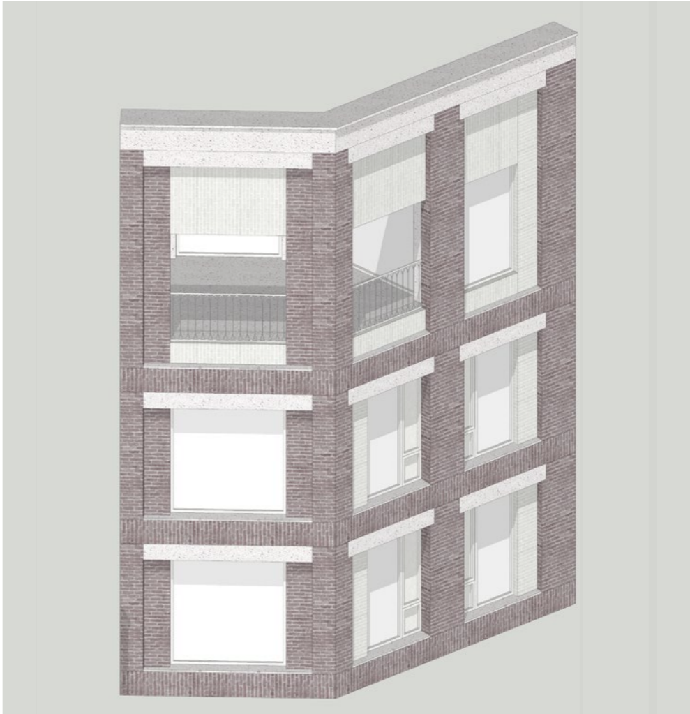
+ Double height expressed openings with a double height expression and thicker pre-cast coping
