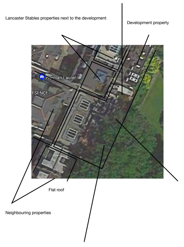
There is space on the flat roof to place any plant a reasonable distance from habitable spaces to minimise the noise and vibration impacting all the adjacent living spaces.
