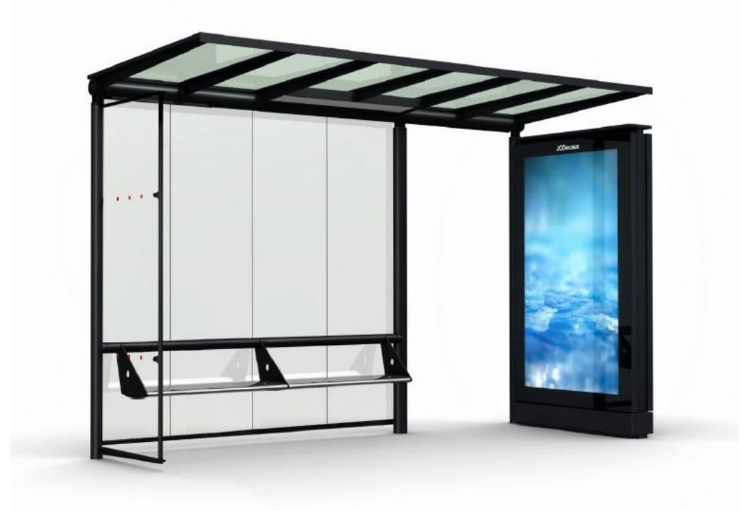
The shelter roof structure is welded steel construction, supporting five panels of toughened laminated glass, which cannot fall in the event of breakage. The glass is specially treated to reduce the heat of the sun rays by more than 50% and is waterproofed through seals fitted in the glazing bars. The shelter roof is gently sloped to drain rainwater behind rear glass.
