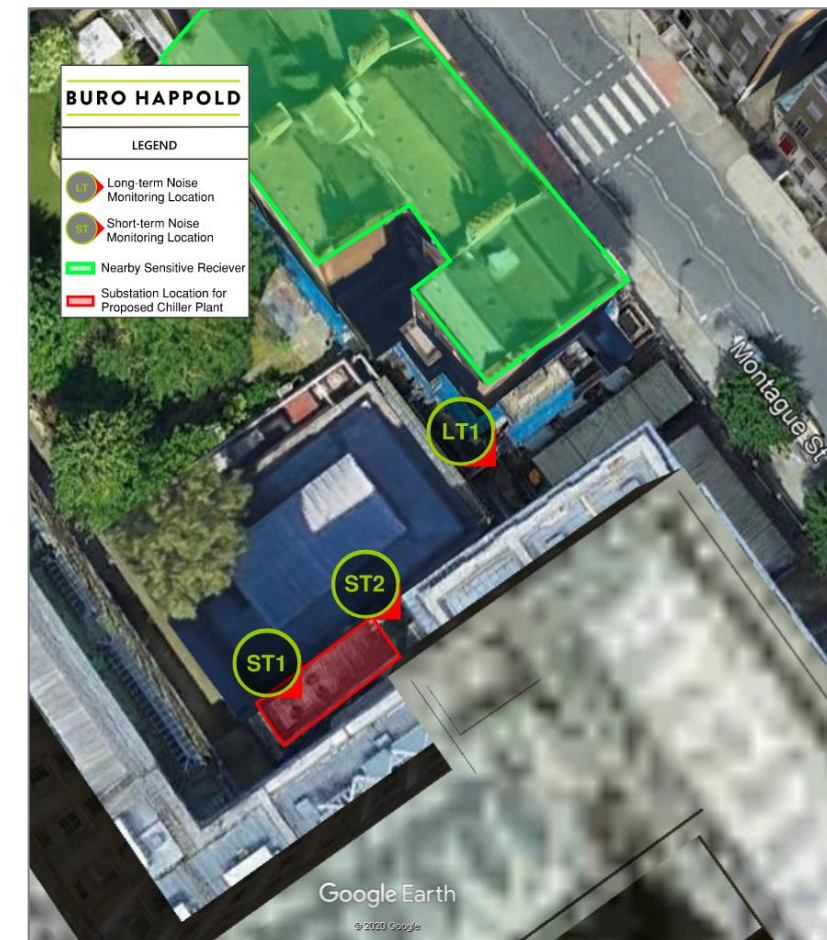
Figure 4—1 Annotated aerial image indicating noise survey measurement locations ST1, ST2 and LT1 (Source: Google Earth, @2020Google).
