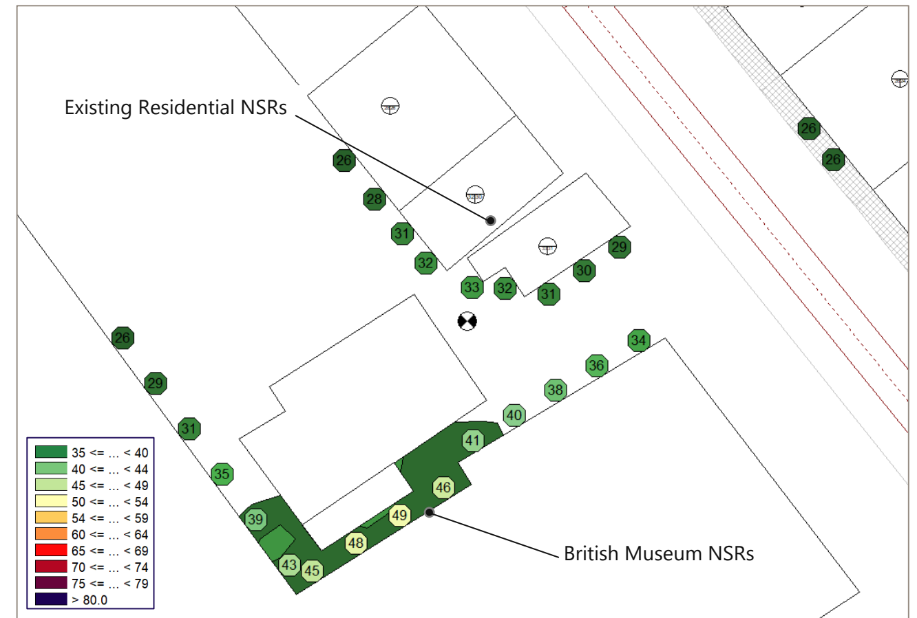
Figure 5—3 Highest calculated L_{A,T,facade} noise levels due to noise emissions from the JKR2490.C5 W3EIEPA(EC)S remote condenser units
