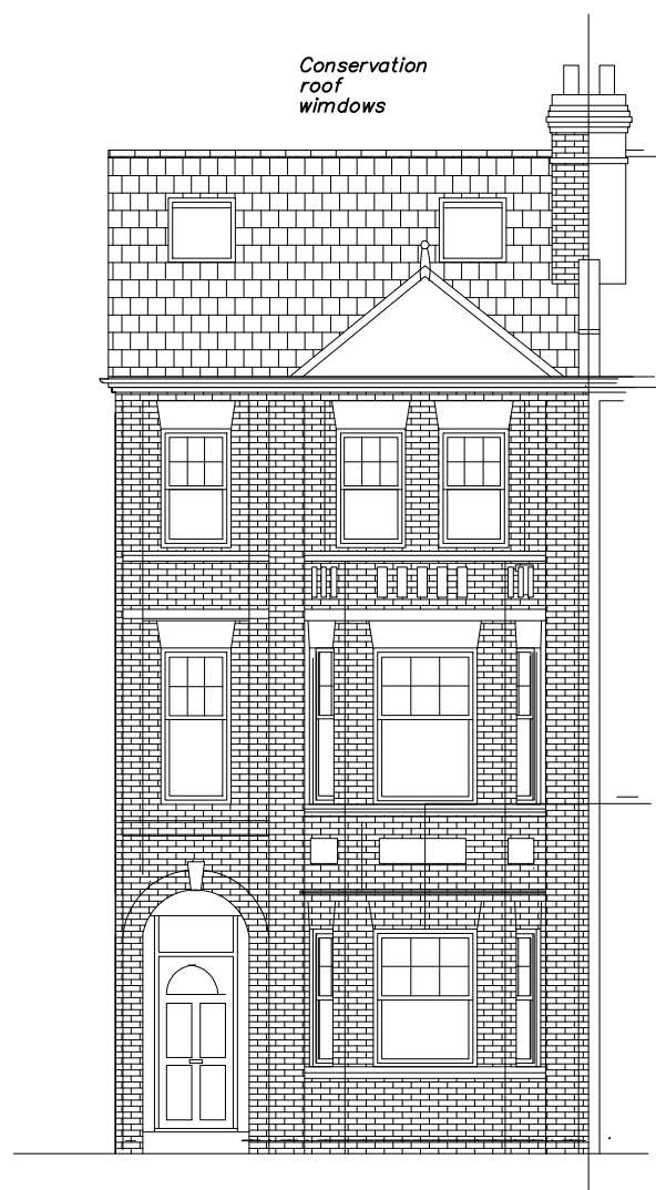
Proposed front elevation Scale 1:100
