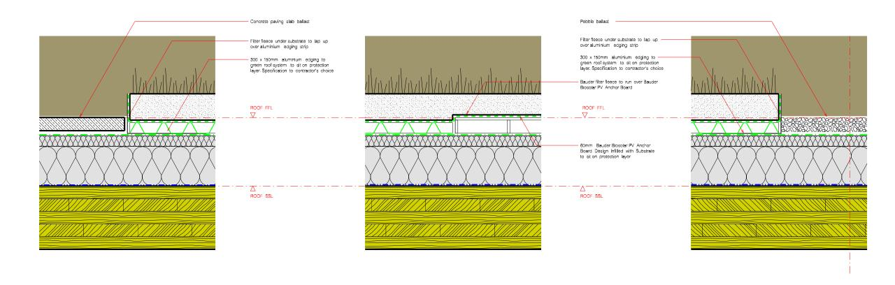
(1) GREEN ROOF TO CONCRETE PAVING SLAB DETAIL
