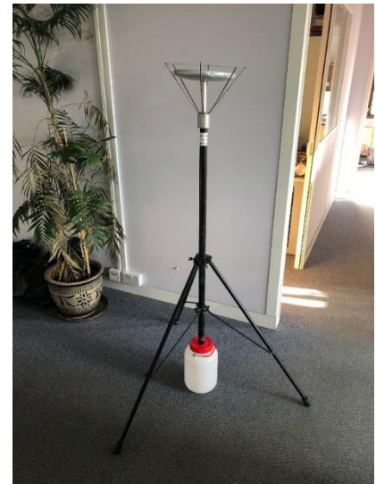
Figure 2: Picture of a settleable dust gauge with collection bottle
