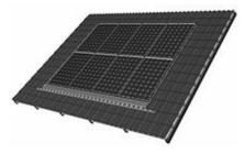
Roof-integrated systems are screwed directly onto the roof batten, replacing a conventional covering. No additional aluminium profiles or roof hooks are required since modules are installed using specially designed bearing elements.
