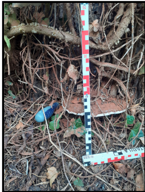
Photo 6: Fungal fruiting body on southern base of tree T02 with probe fully inserted to left.
