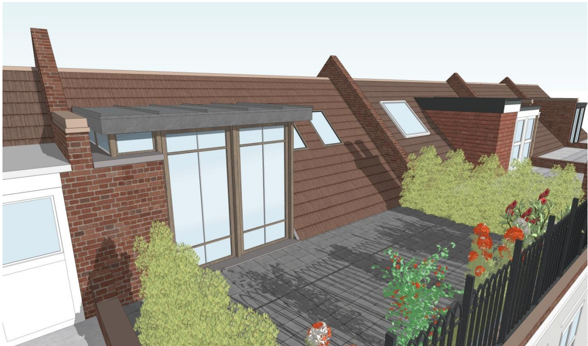
fig. 9: Perspective of proposed enlarged rear dormer and dormers at nos. 15C and 19C Swain's Lane.
