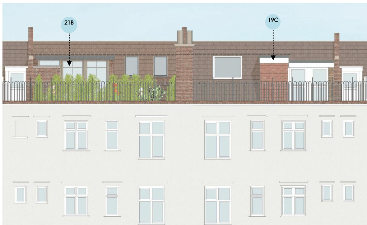
fig. 8: Rear elevation close-up demonstrating a dormer height lower to that of no. 19C Swain's lane.
