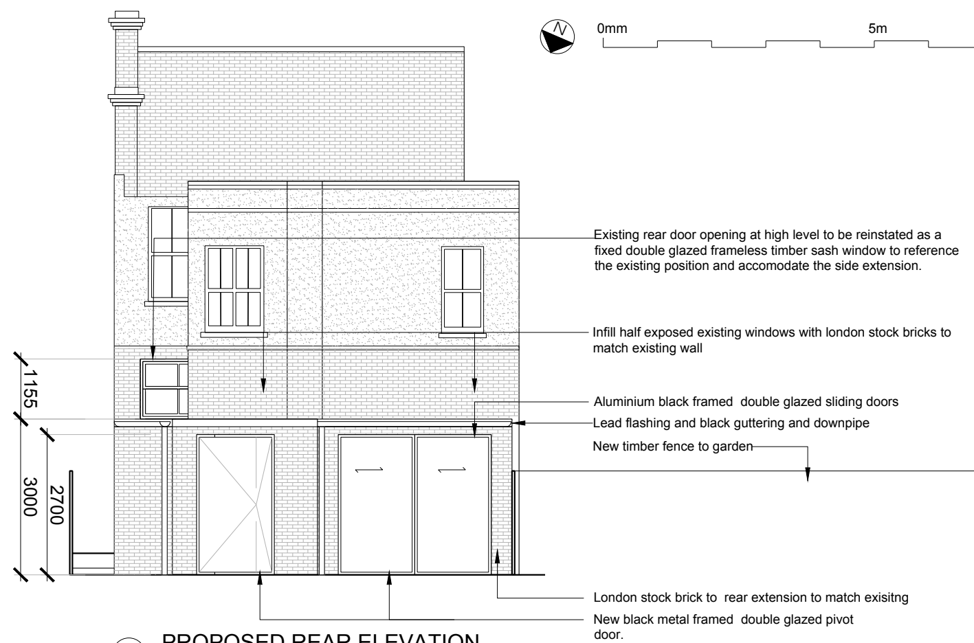
3 PROPOSED REAR ELEVATION Scale: 1:100
