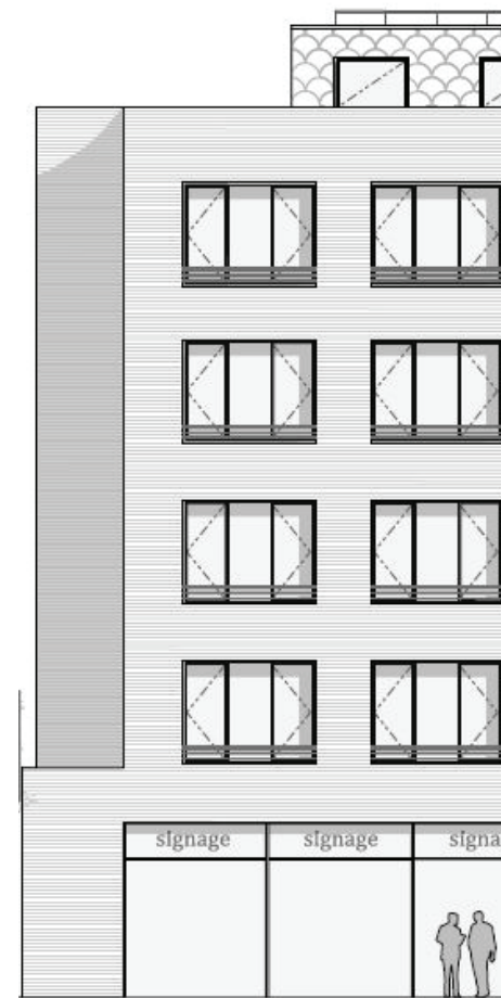
Extract of Approved Drawing Front Elevation Showing Green Scallop Ceramic Tiles to Top Setback
