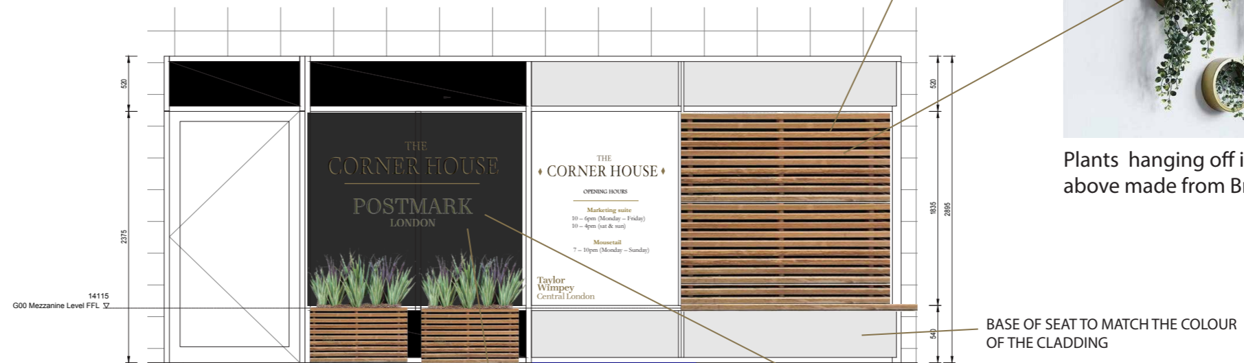
FULL WINDOW VINYL WITH METALLIC GOLD/BLACK WRITING TO COVER THE TV SCREEN JOINERY BEHIND
